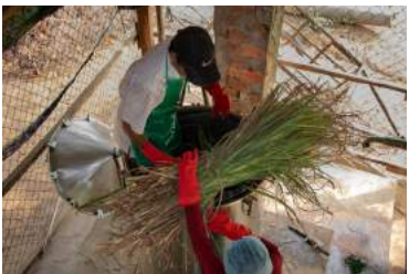
Step 2.2 : filling of the distillation tank
